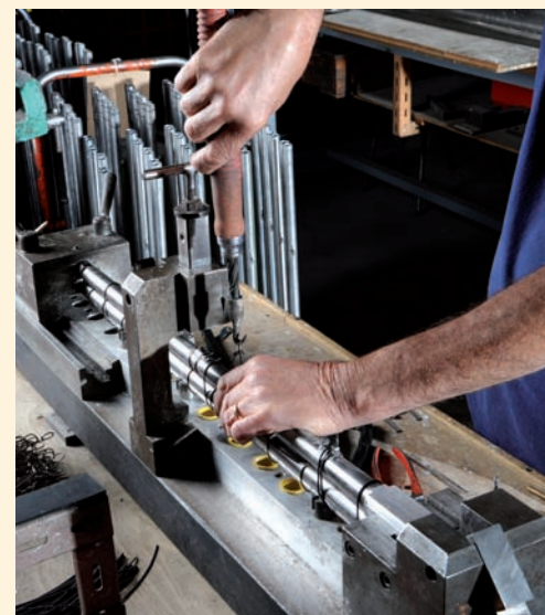
Assembly of barrels before welding in 2014
